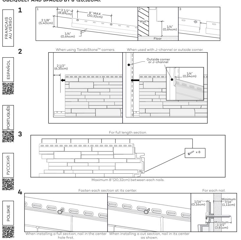
Install sections and space equally. For installation when outside temperature is between 30°F(-1°C) and 5 100°F(38°C), press against previous section. Between 30°F(-1°C) and 100°F(38°C) Below 30°F(-1°C) Leave 1/16"(0,16cm)
