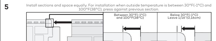
Below 30°F(-1°C), position the section slightly right (1/16"(0,16cm)) previous section.
