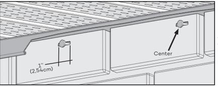
If you need to attach a section in an area other than the installation hole, create a 1"(2,54cm) long slot to allow nailling. Always nail in the middle of the slot.
